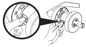
Insert the key into the outside lever and turn it 90° degree clockwise. Push the outside lever onto the chassis until the catch engages in lever.
