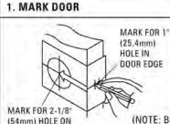
Start approximately 36" (914mm) from floor, Fold and apply template to edge of door and mark center of door edge as indicated on template. Mark centerhole on door face through guide on template.
